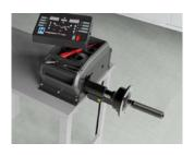
Version with minimal size to secure to a workbench with two support brackets (ideal for both workshop and for mobile service)
